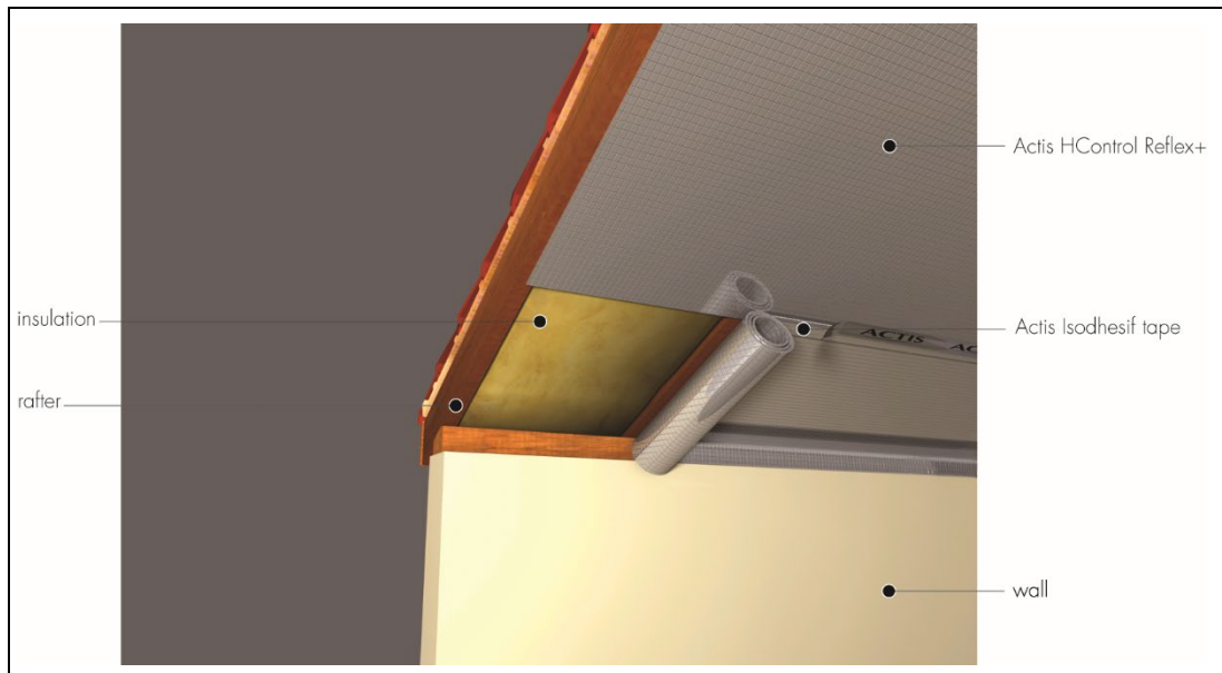
Figure 2 Roof installation with one unventilated air gap
